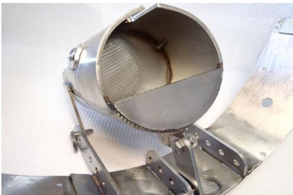
**Fig. 1** Screened Inline Flow-Through (SIFT) sediment trap
