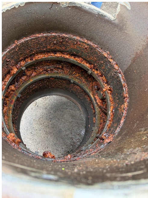
Left: Mineral buildup inside the 24" valve.
