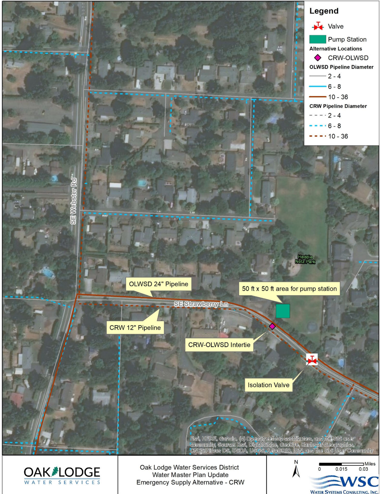
Figure 5-2. Proposed Concept for Emergency Intertie with CRW
