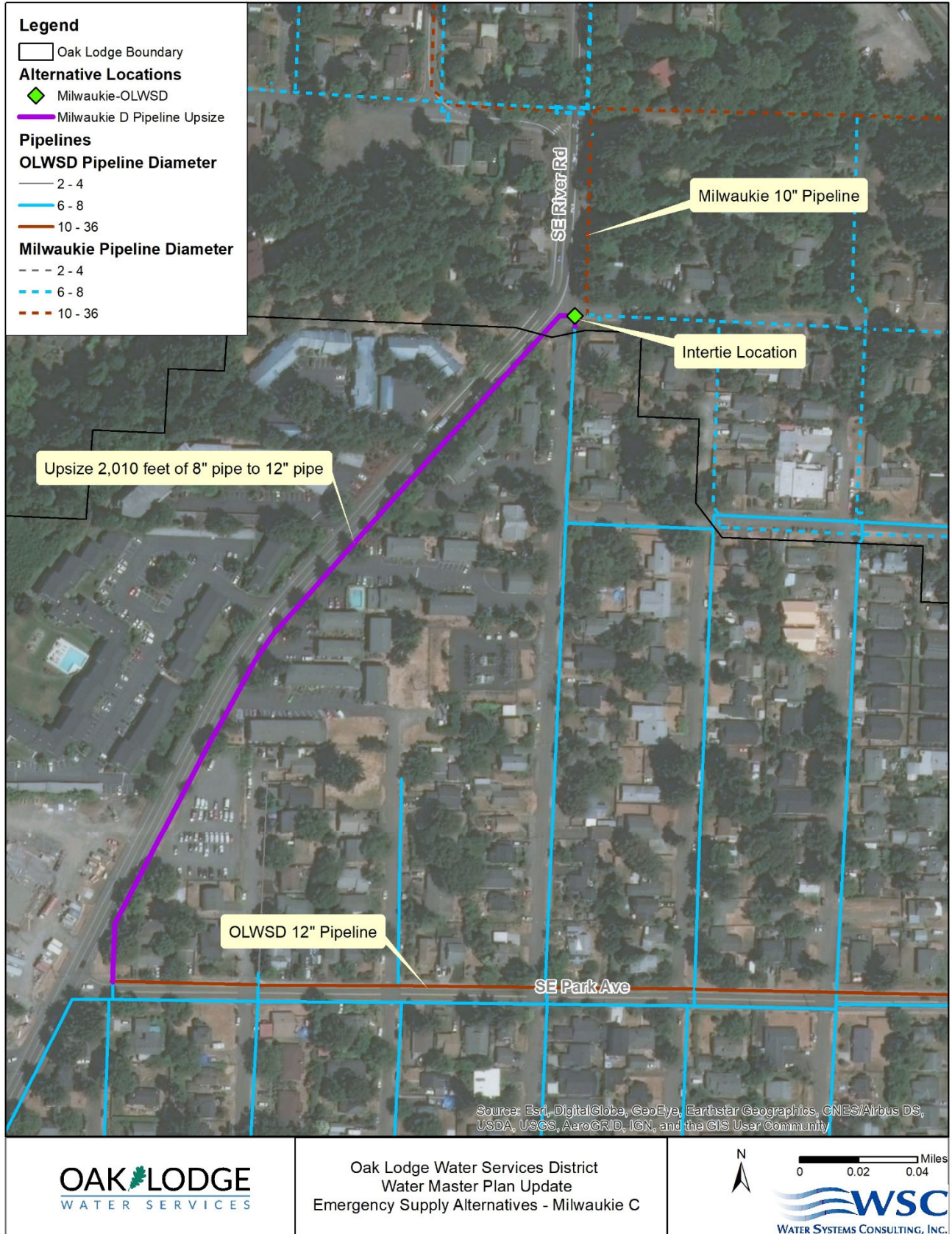
Figure 5-3. Proposed Concept for Emergency Intertie with the City of Milwaukie
