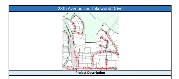
This project replaces 4015 feet of 8-inch cast iron pipe with 8 and 12-inch ductile iron pipe. It will also create a loop in the system where the District has had to flush more often to keep the water fresh tasting.
