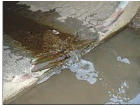
Low Severity Suds Rating: 1 Note: Suds do not appear to travel; very thin foam layer
