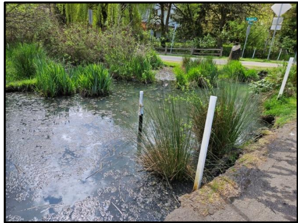
Photo 3: Water level logger installed upstream of Boardman Avenue.
