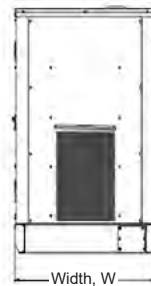
Sound Attenuated Enclosure on Skid Base
