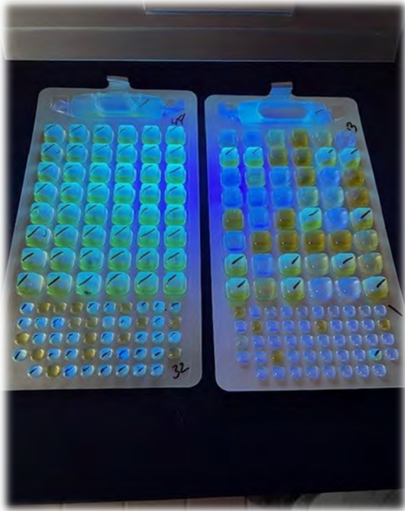
Failed E. Coli test (Left) and the retest (right)
