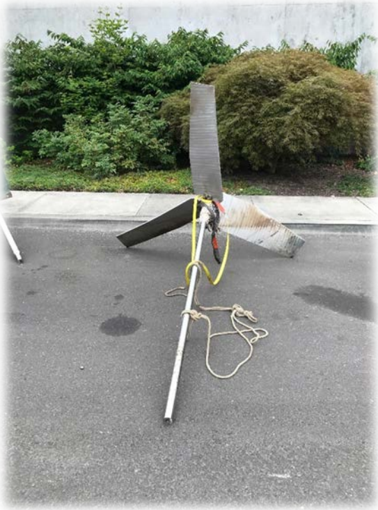
Photo 5 Blade and broken shaft
